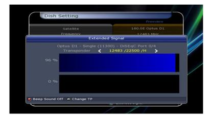
Move the dish until you get a lock on the satellite (Quality will show red). This step may take some time. You should now optimize the Elevation and Azimuth of your dish and the Skew of the LNB to get the Quality indicator as high as possible. Your receiver is pre tuned so once you have finished you can just press exit a few times and proceed to watch TV.
