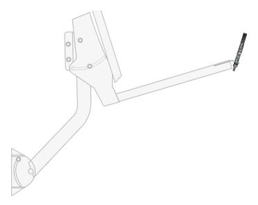
Then install the new 40mm throat LNB with the skew shown in its installation instructions and reconnect the cable.
