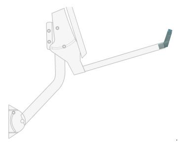
Replace it with the conversion kit, it will bolt against the top internal surface of the rectangular arm that holds the LNB.
