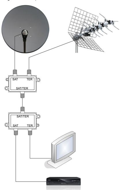
The SAT/TER diplexers allow the STB to provide power to the LNB but do not allow power to be passed on the terrestrial side. If you wish to use a masthead amplifier with the UHF aerial you must put the power injector between the Masthead amplifier and the first SAT/TER diplexer.
