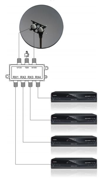
In this example you need to configure the STBs so that only Horizontally polarized channels are scanned in on the OPTUS D1 satellite and only Vertically polarized channels are scanned in on the OPTUS D2 satellite. If both polarities are required on a single satellite Dual Output LNBs may be used.
