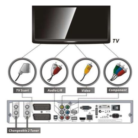
NOTE : HDMI or component (YPbPr) is recommended for Digital TVs. The SCART cable connection is recommended for analogue TVs or VCRs The composite connection(RCA cable) is recommended for analogue TVs You cannot view high definition video with the SCART and the composite video connector.
