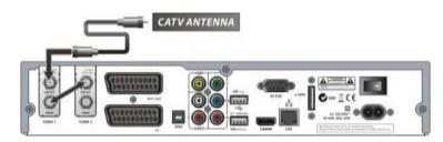
• Connecting one cable to each Tuner
