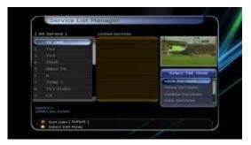
• Move Services : All service lists will be shown on left side of the window, services to be moved will be shown on the middle window. Move the service to the middle window by using the ARROW and OK buttons, then the middle window service will be moved to a specified location when the desired location is selected from the left window.
