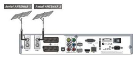
5.3 In case of C + C (Cable + Cable) tuners
