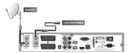
5.6 In case of T(T2) + C (Terrestrial + Cable) tuners
