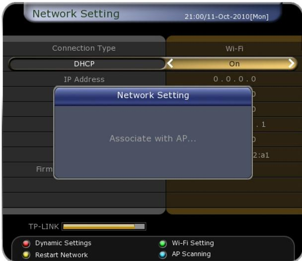
If DHCP is enabled the DHCP server will assign an IP Address to the Ultraplus. The DHCP server may be a function of the Access Point or Router.
