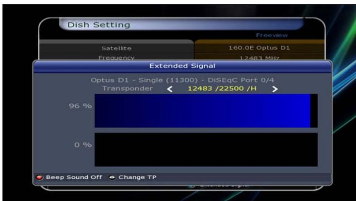
Move the dish until you get a lock on the satellite (Quality will show red). This step may take some time. You should now optimise the Elevation and Azimuth of your dish and the Skew of the LNB to get the Quality indicator as high as possible. Your receiver is pre tuned so once you have finished you can just press exit a few times and proceed to watch TV.
